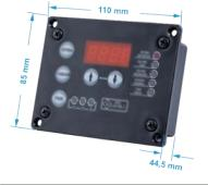
Showing the difference between external pressure and internal pressure on the screen, it gives pressure information. External pressure info is delivered to the sensor within the unit via pneumatic hose and it shows the difference with internal pressure on the screen. It gives audio and visual warning under the adjusted pressure value. It has black out mode, alarm muting, built-in test features. Requested pressure difference warning can be adjusted manually.
