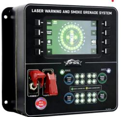
**AFSS SGS-3 Control Unit** is a control unit which can automatically control laser and smoke grenade systems.
